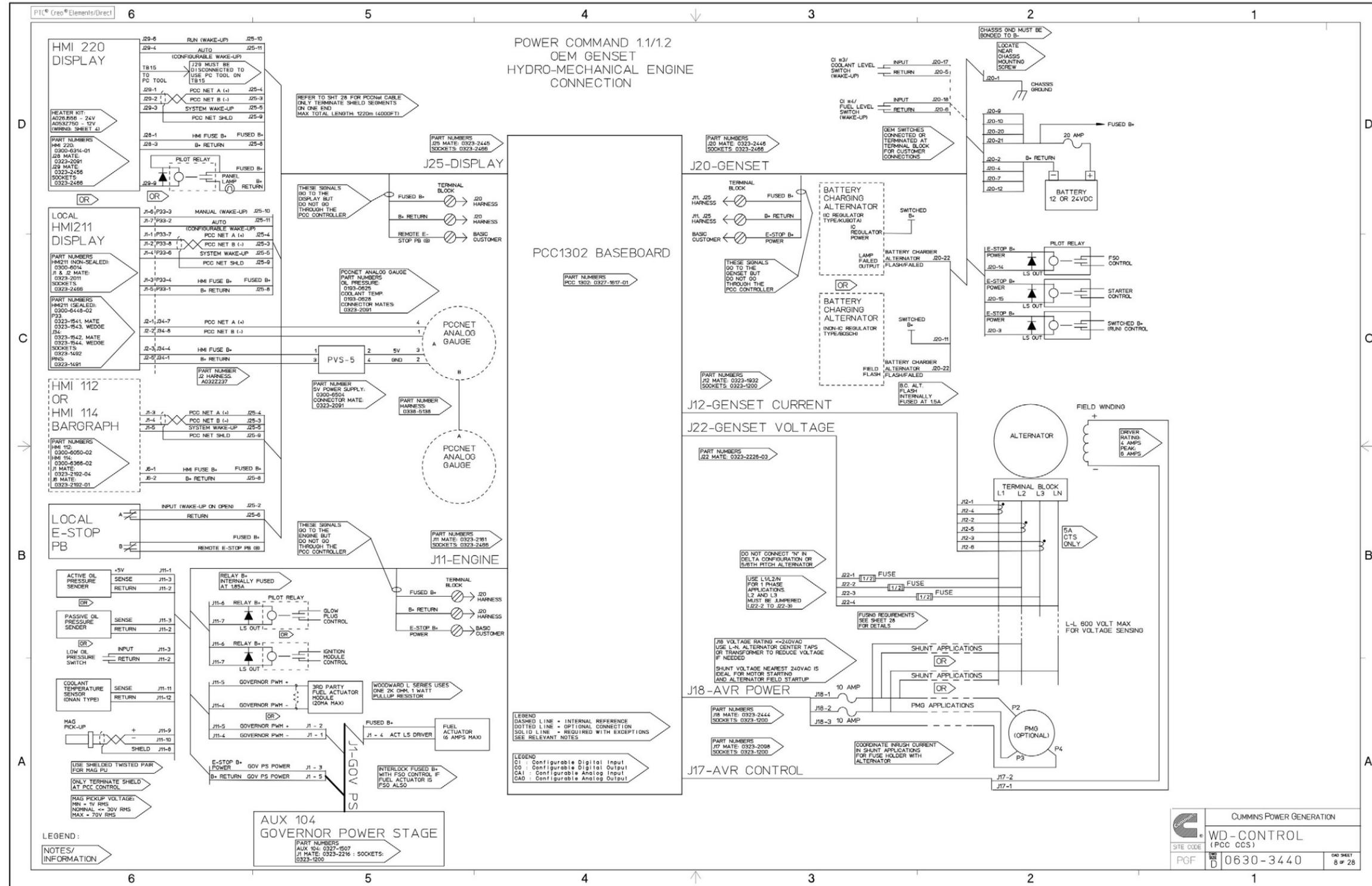
FIGURE 83. PC 1.1 CONTROL WIRING DIAGRAM (SHEET 2 OF 4)
