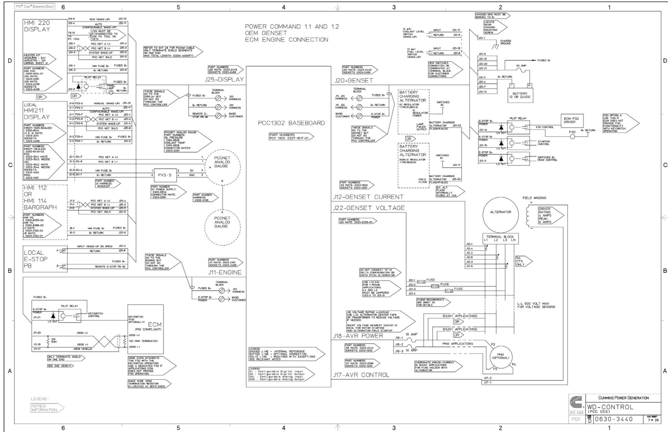
FIGURE 82. PC 1.1 CONTROL WIRING DIAGRAM (SHEET 1 OF 4)
