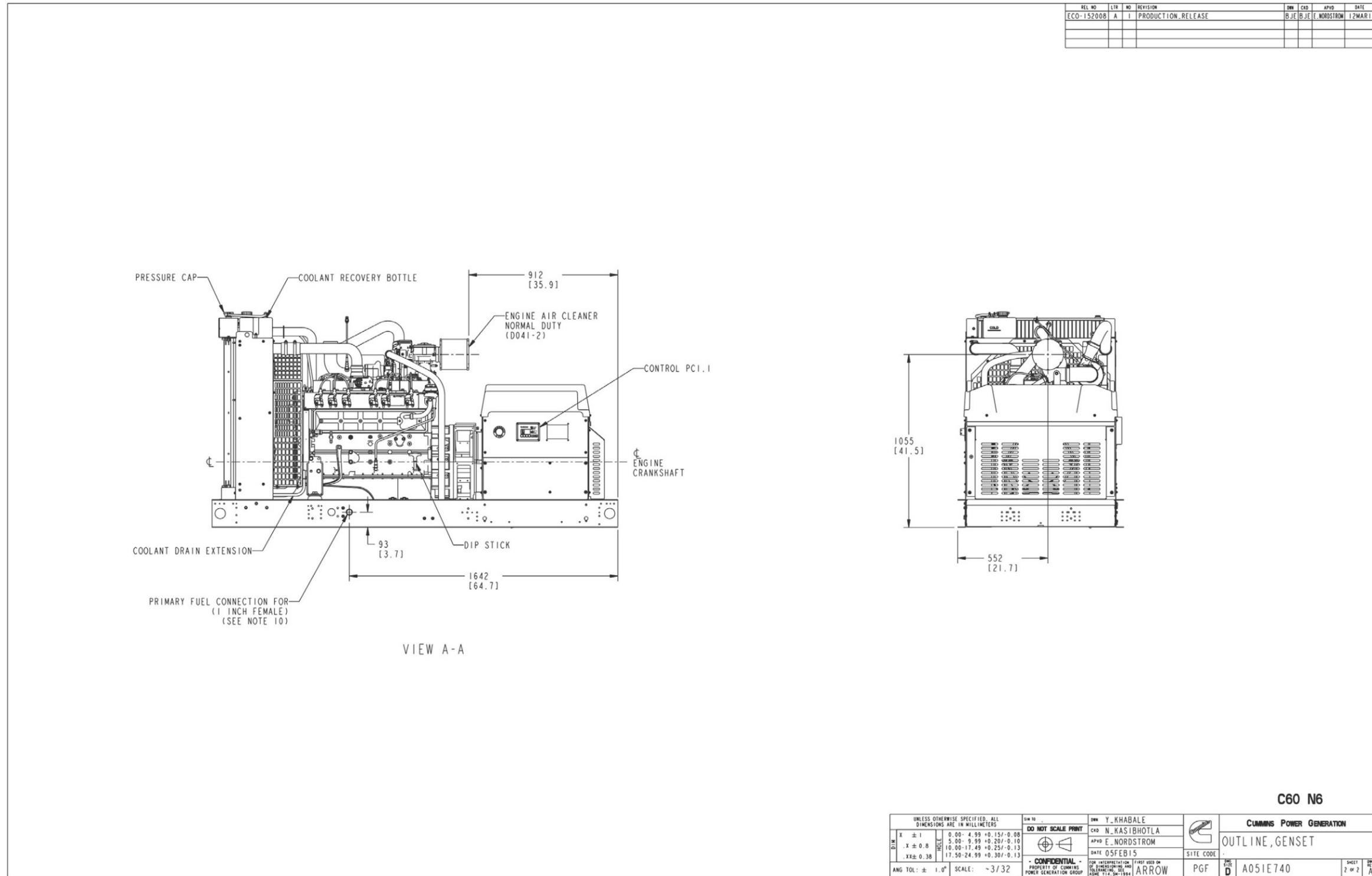
FIGURE 36. GENERATOR SET OUTLINE, 60 KW (SHEET 2 OF 2)
