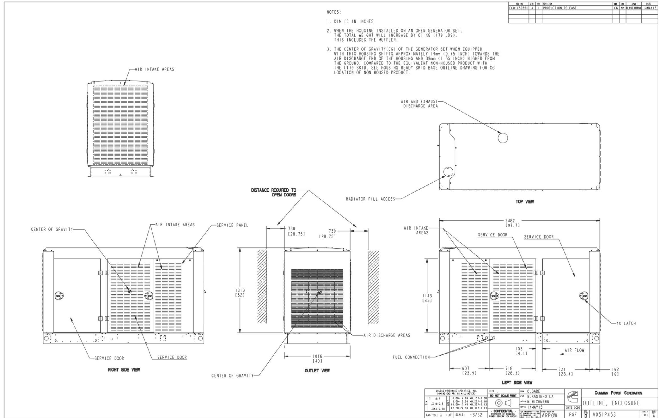
FIGURE 42. ENCLOSURE OUTLINE, WEATHER (SHEET 1 OF 1)
