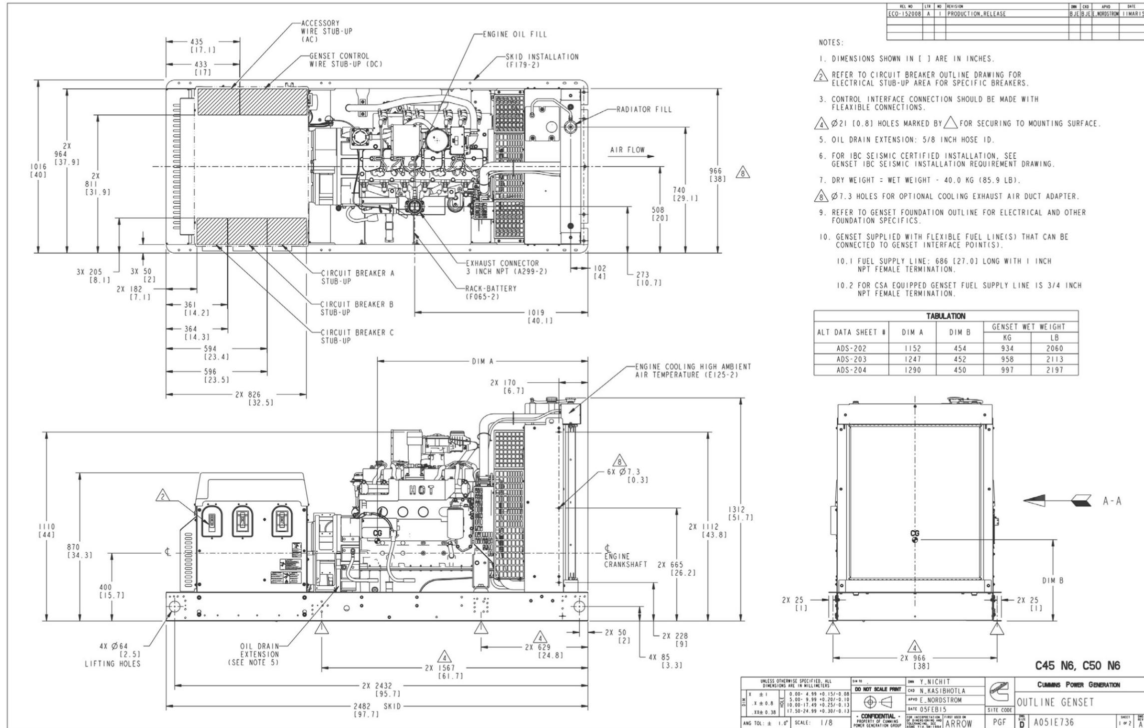
FIGURE 33. GENERATOR SET OUTLINE, 45-50 KW (SHEET 1 OF 2)
