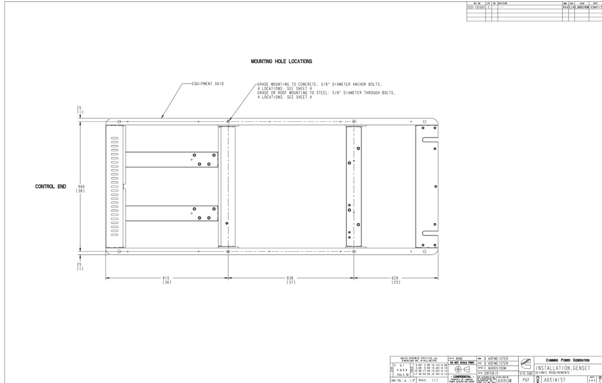
FIGURE 91. SEISMIC INSTALLATION REQUIREMENTS (SHEET 3 OF 4)
