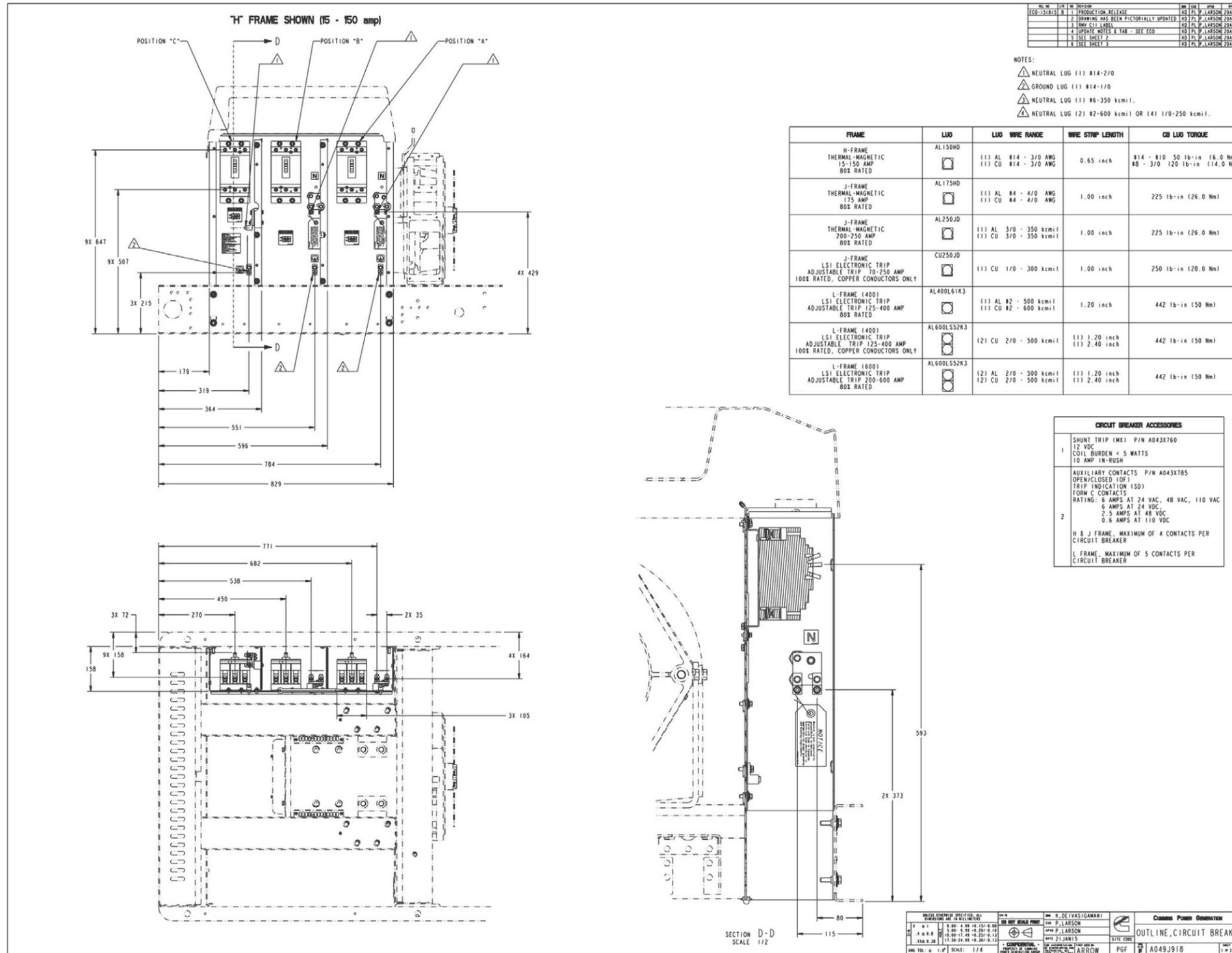
FIGURE 73. CIRCUIT BREAKER OUTLINE (SHEET 1 OF 3)
