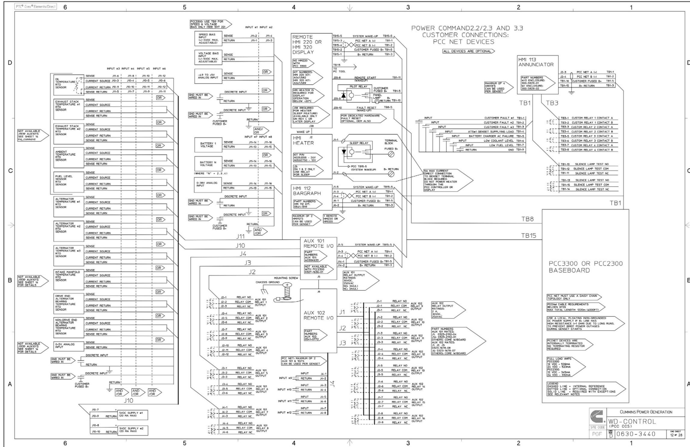
FIGURE 87. PC 2.3 CONTROL WIRING DIAGRAM (SHEET 2 OF 3)
