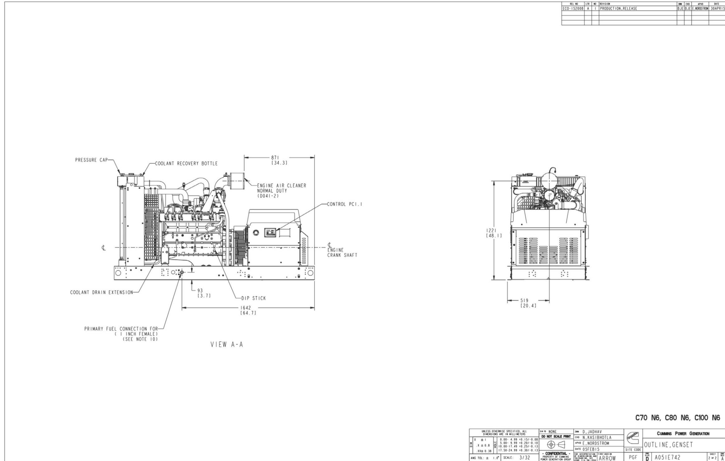
FIGURE 38. GENERATOR SET OUTLINE, 70-100 KW (SHEET 2 OF 2)
