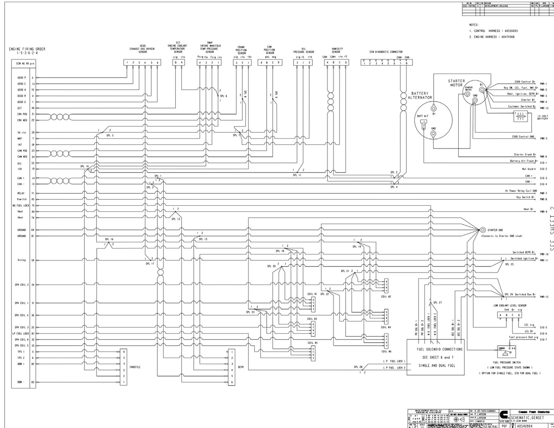
FIGURE 66. WIRING DIAGRAM FOR PCC 2300 (90 PIN ECM) (SHEET 1 OF 7)
