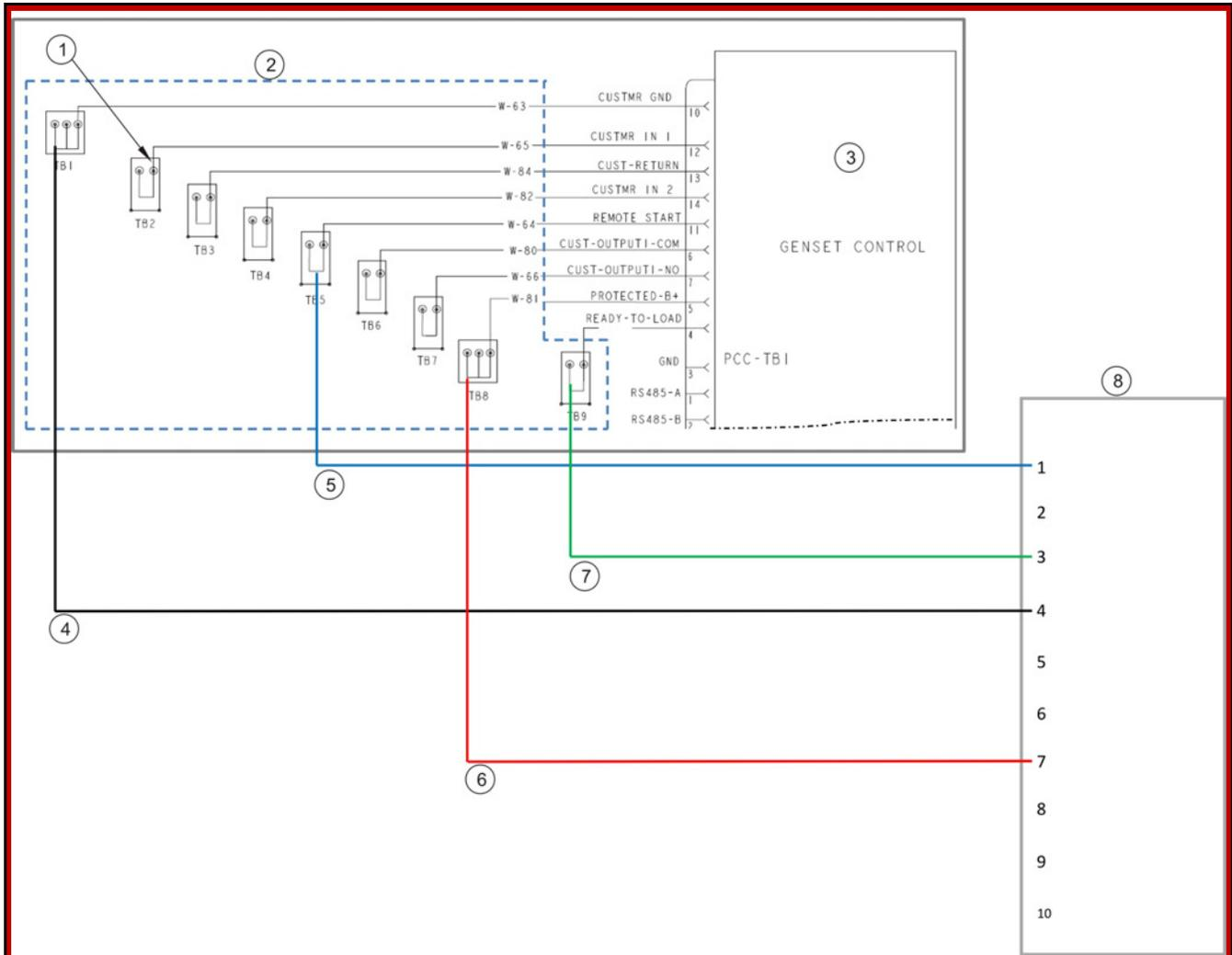
**FIGURE 12. GENERATOR SET TO RA TRANSFER SWITCH DC CUSTOMER CONNECTIONS**
