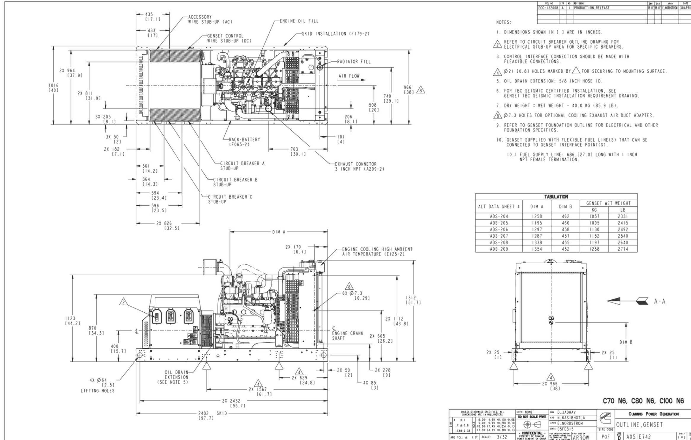
FIGURE 37. GENERATOR SET OUTLINE, 70-100 KW (SHEET 1 OF 2)
