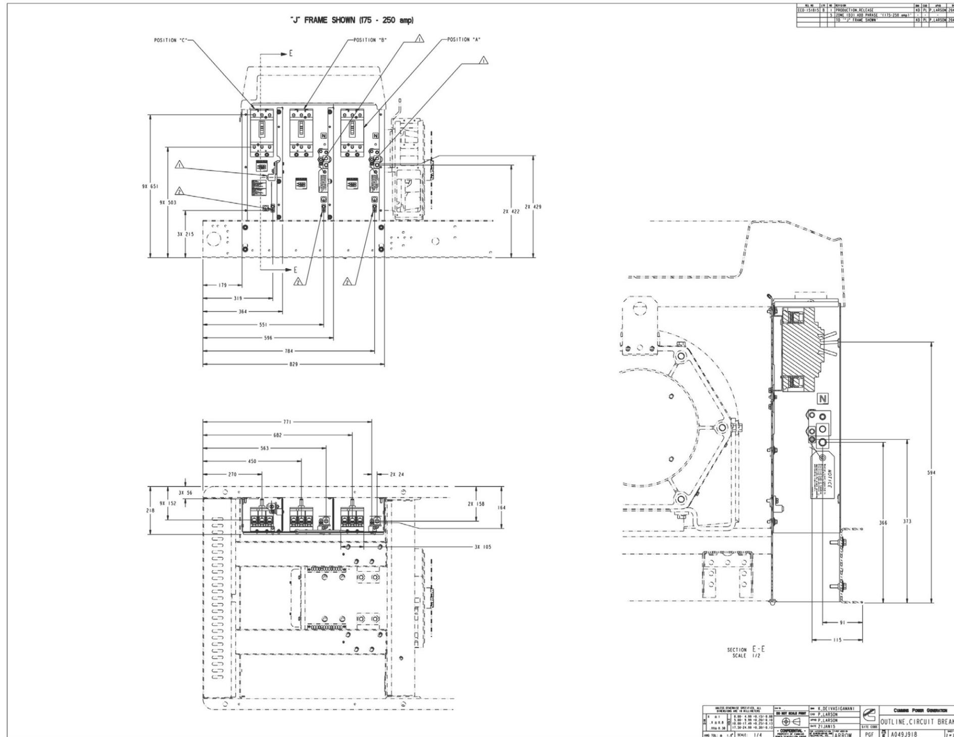
**FIGURE 74. CIRCUIT BREAKER OUTLINE (SHEET 2 OF 3)**
