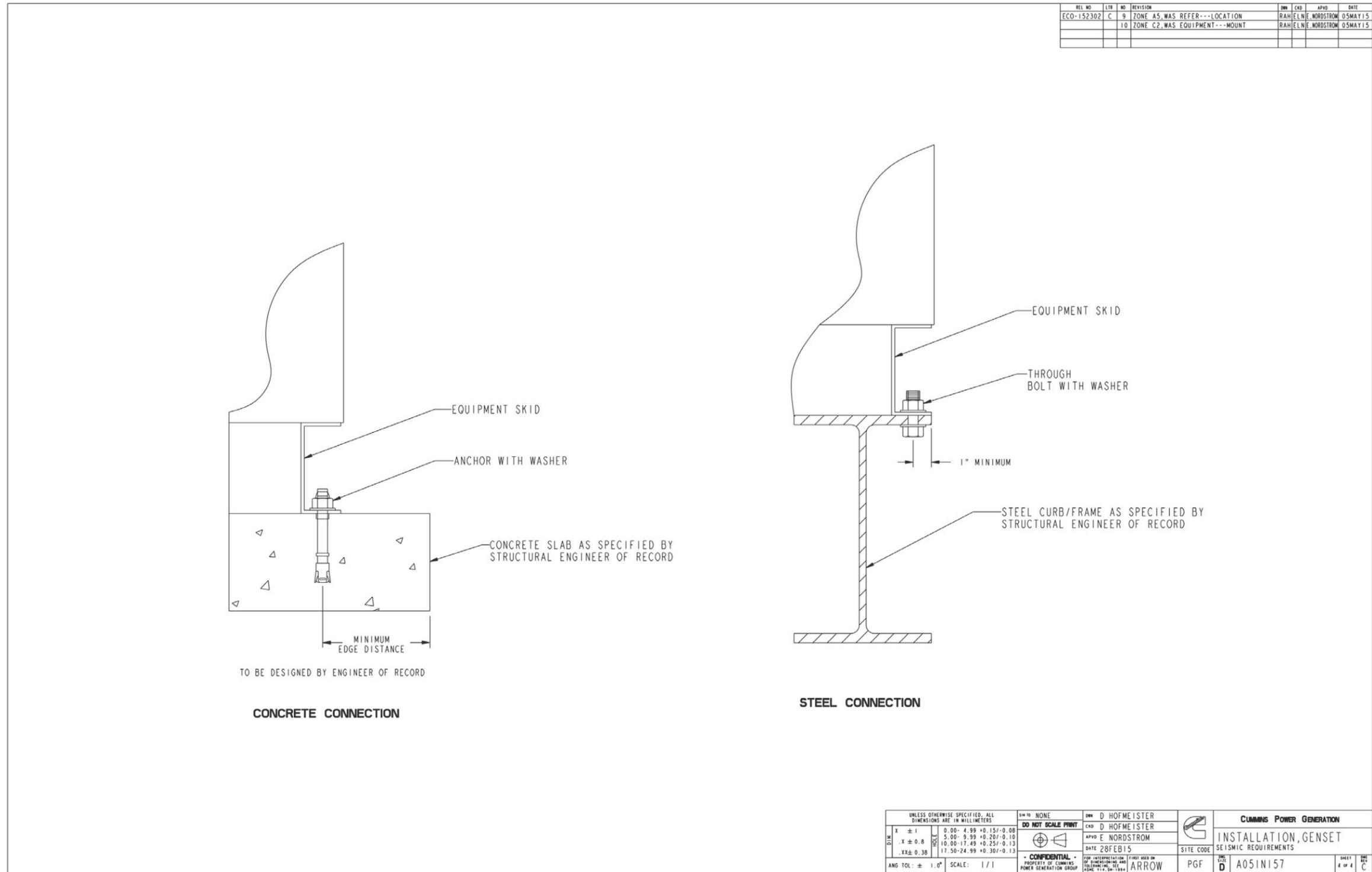
FIGURE 92. SEISMIC INSTALLATION REQUIREMENTS (SHEET 4 OF 4)
