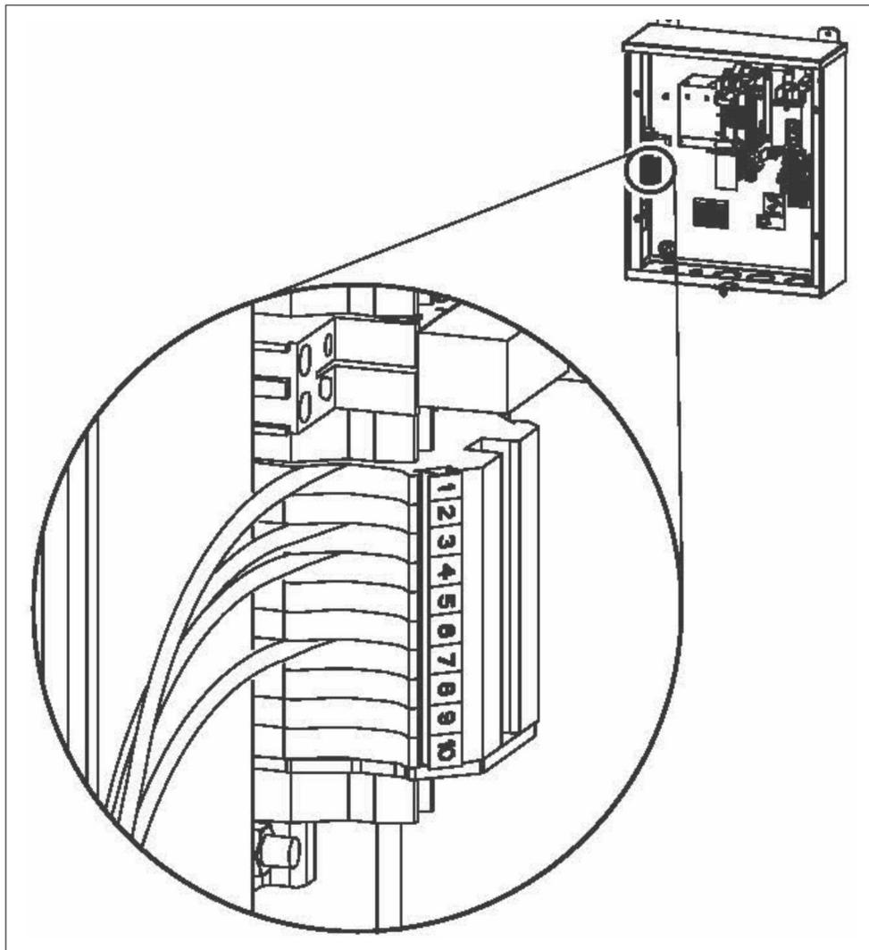
**FIGURE 11. RA SERIES TRANSFER SWITCH DC CONNECTIONS LOCATION**
