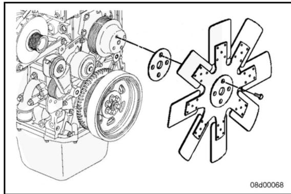
**FIGURE 11. EXAMPLE OF FAN PULLEY REMOVAL**
