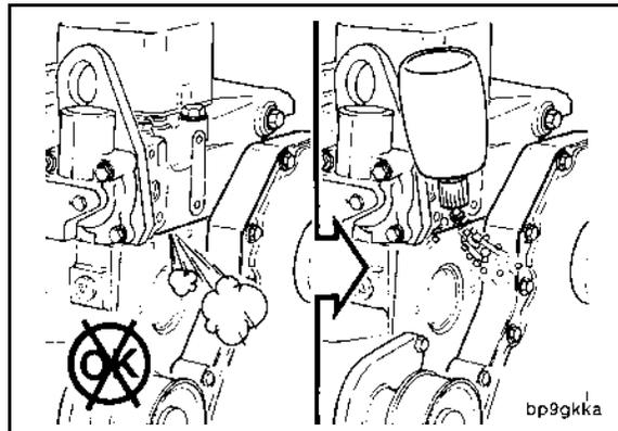
**FIGURE 88. USE LIQUID SOAP TO DETERMINE IF THERE IS A LEAK**
