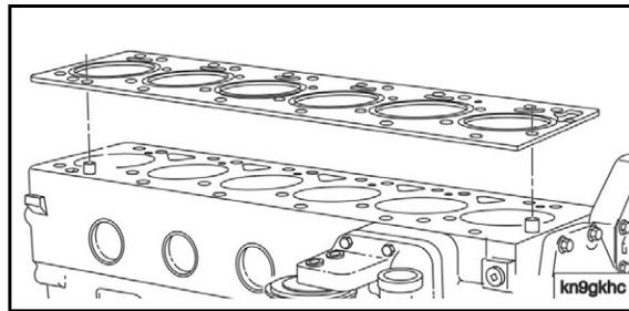
FIGURE 90. REPLACE THE HEAD GASKET
