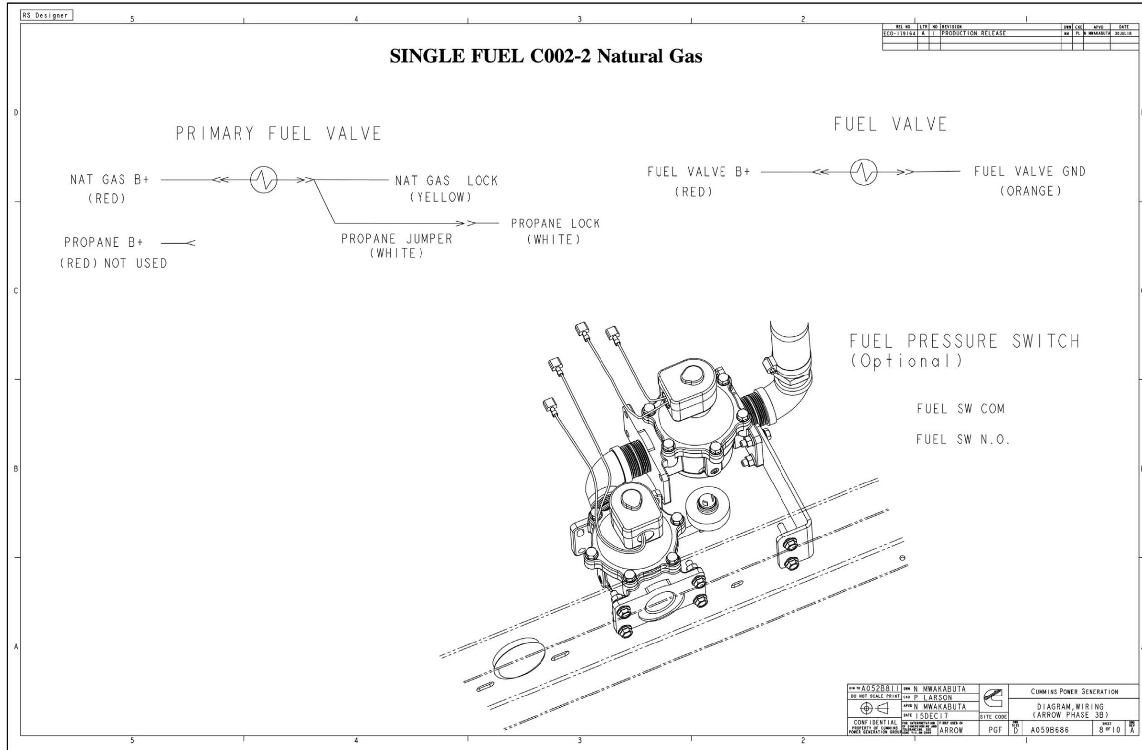
FIGURE 106. WIRING DIAGRAM PC 3.3 (SHEET 8 OF 10)
