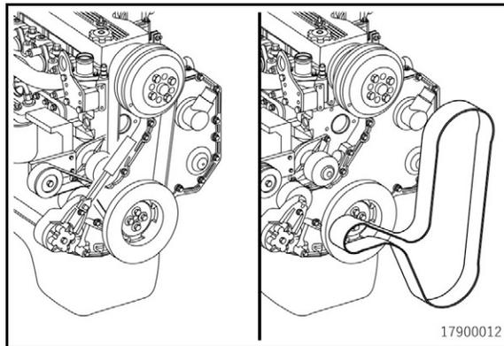
FIGURE 6. LIFT THE TENSIONER
