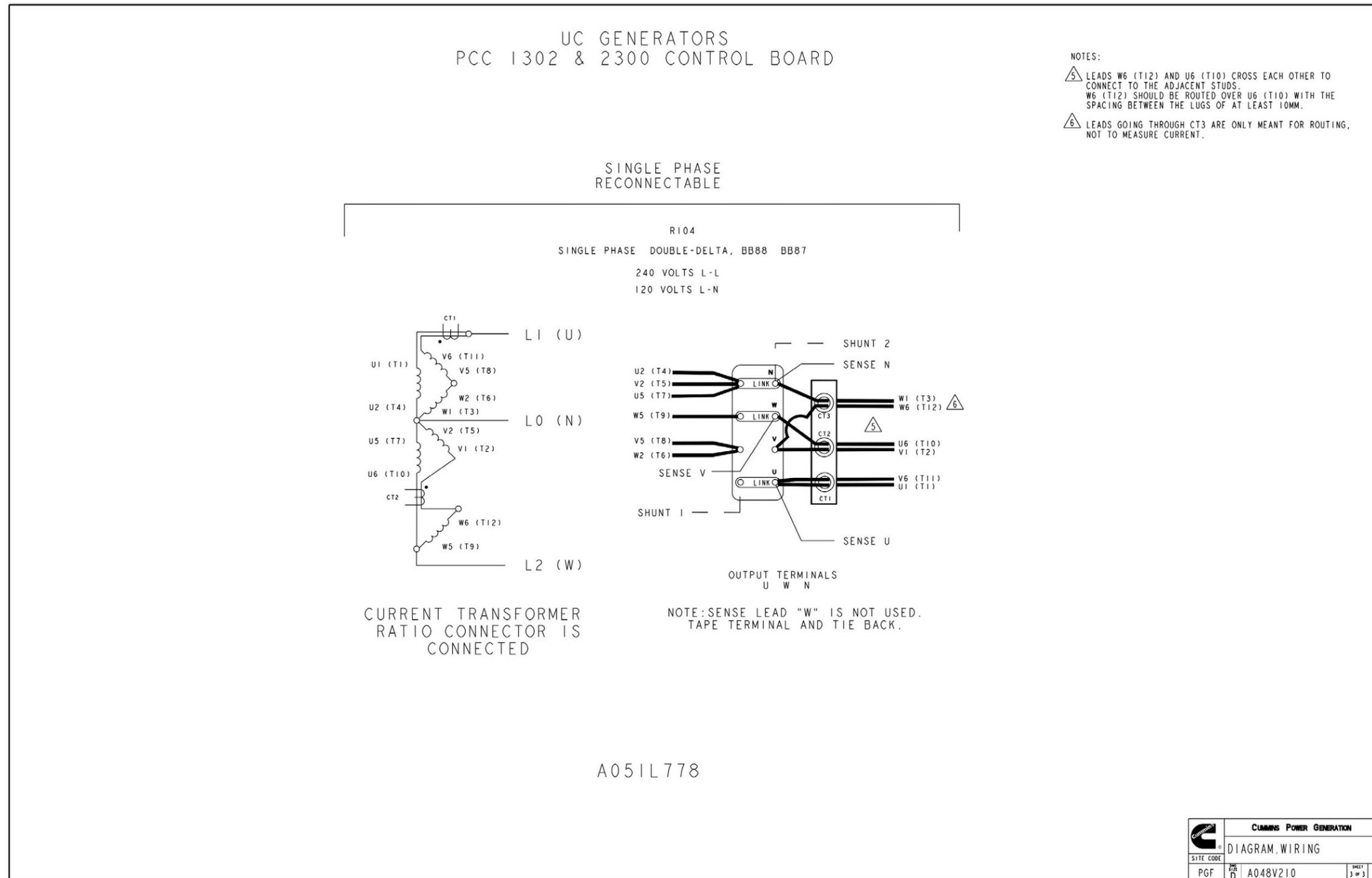
FIGURE 118. RECONNECT DRAWING FOR UC ALTERNATOR (SHEET 3 OF 3)
