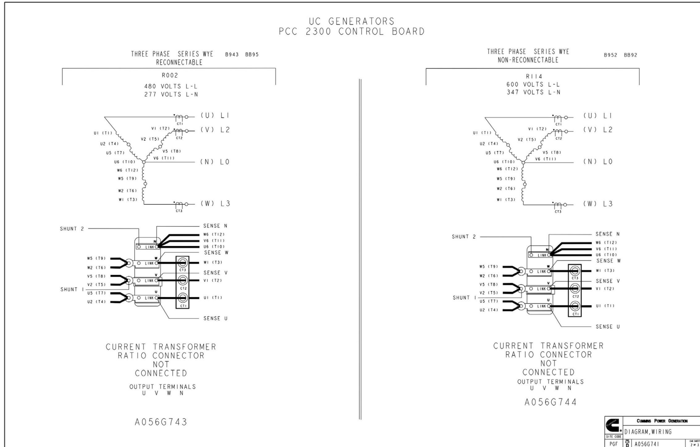
FIGURE 120. RECONNECT DRAWING FOR UC ALTERNATOR (SHEET 2 OF 3)
