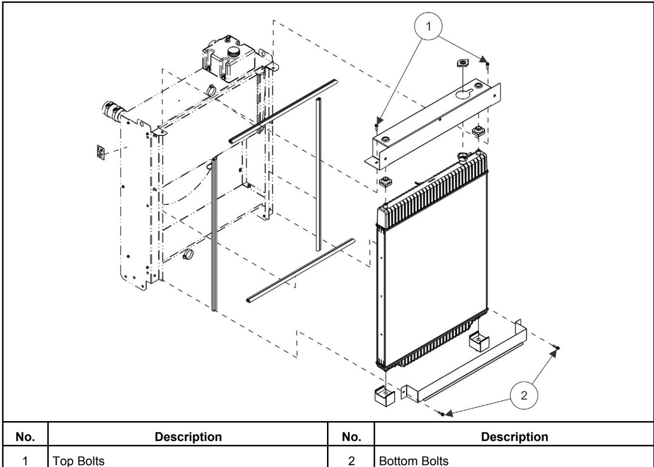
**FIGURE 45. REMOVE THE TOP TWO BOLTS**
