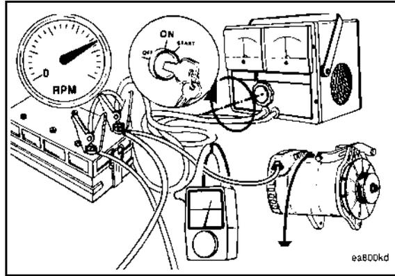
**FIGURE 85. APPLY THE MAXIMUM RATED AMPERAGE LOAD**
