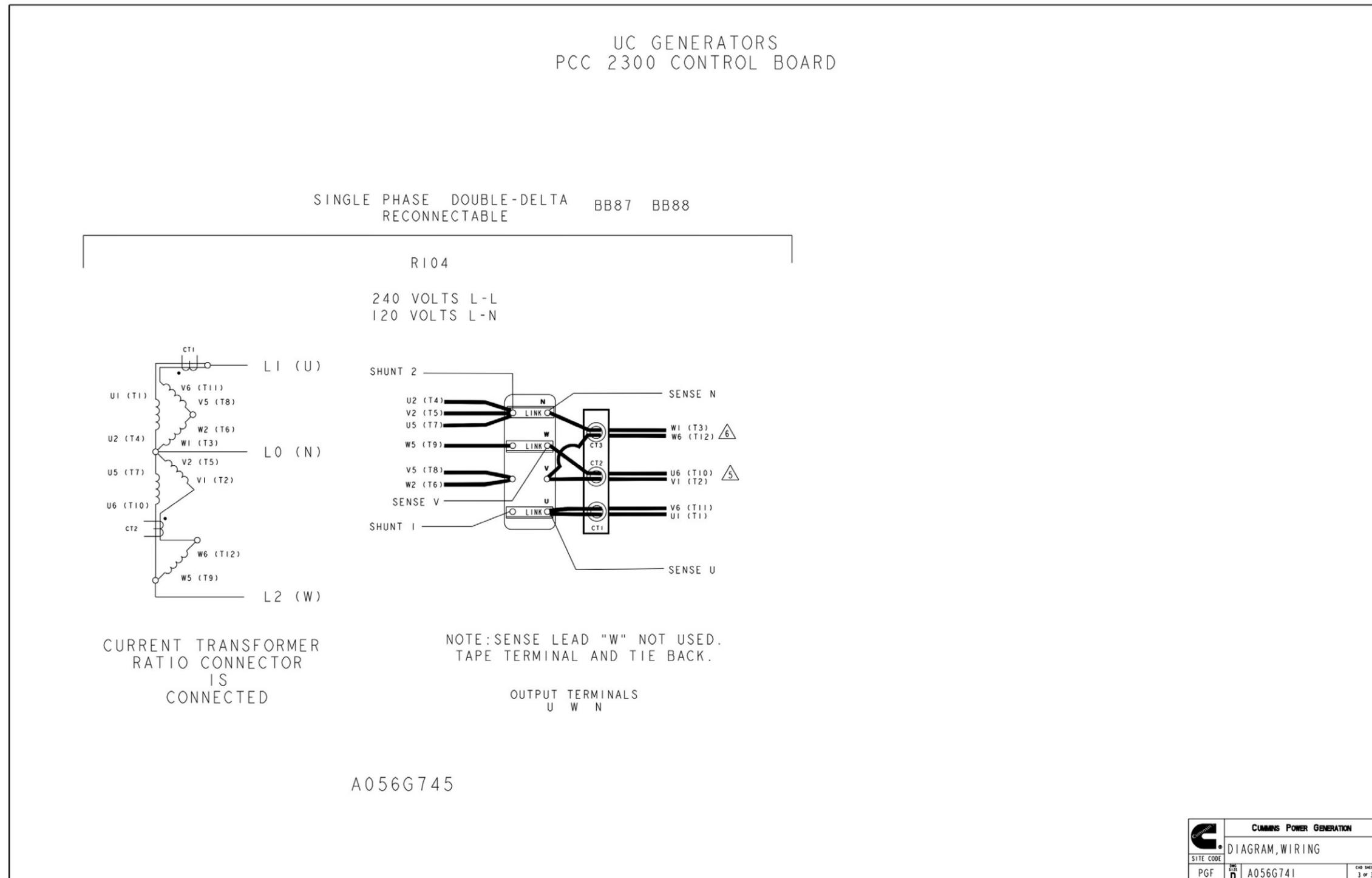
FIGURE 121. RECONNECT DRAWING FOR UC ALTERNATOR (SHEET 3 OF 3)
