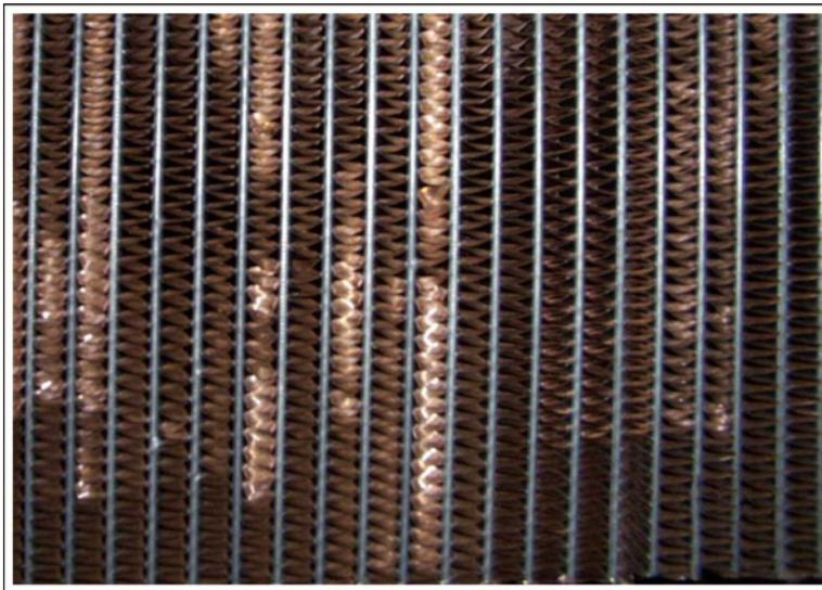
**FIGURE 7. FINS DAMAGED BY PRESSURE WASHING AT ACUTE ANGLES TO CORE FACE**
