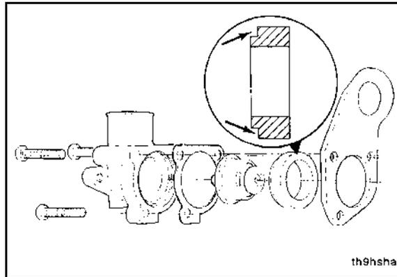
**FIGURE 72. POSITION THE RUBBER SEAL**
