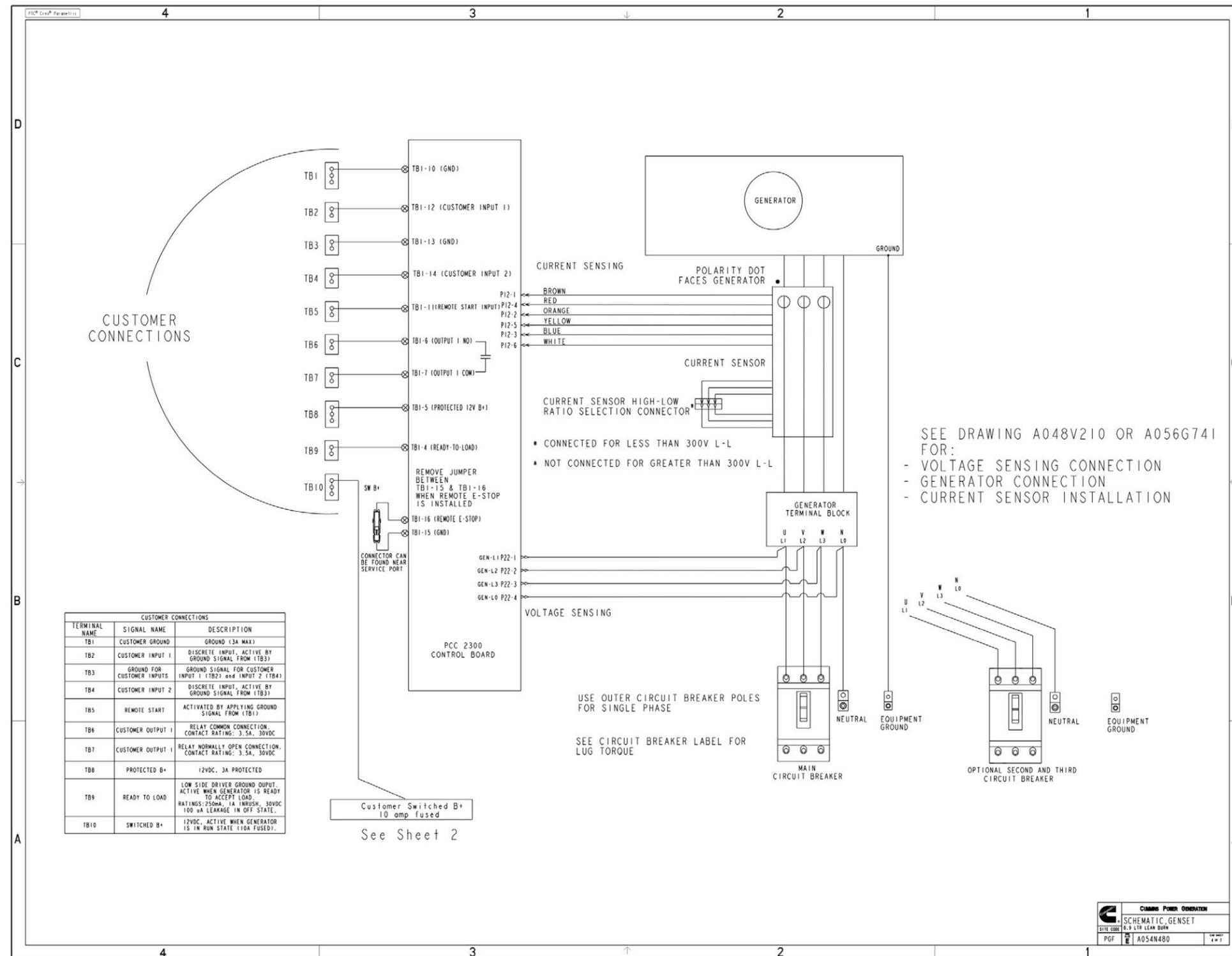
FIGURE 95. WIRING DIAGRAM PC 2.3 (SHEET 4 OF 7)
