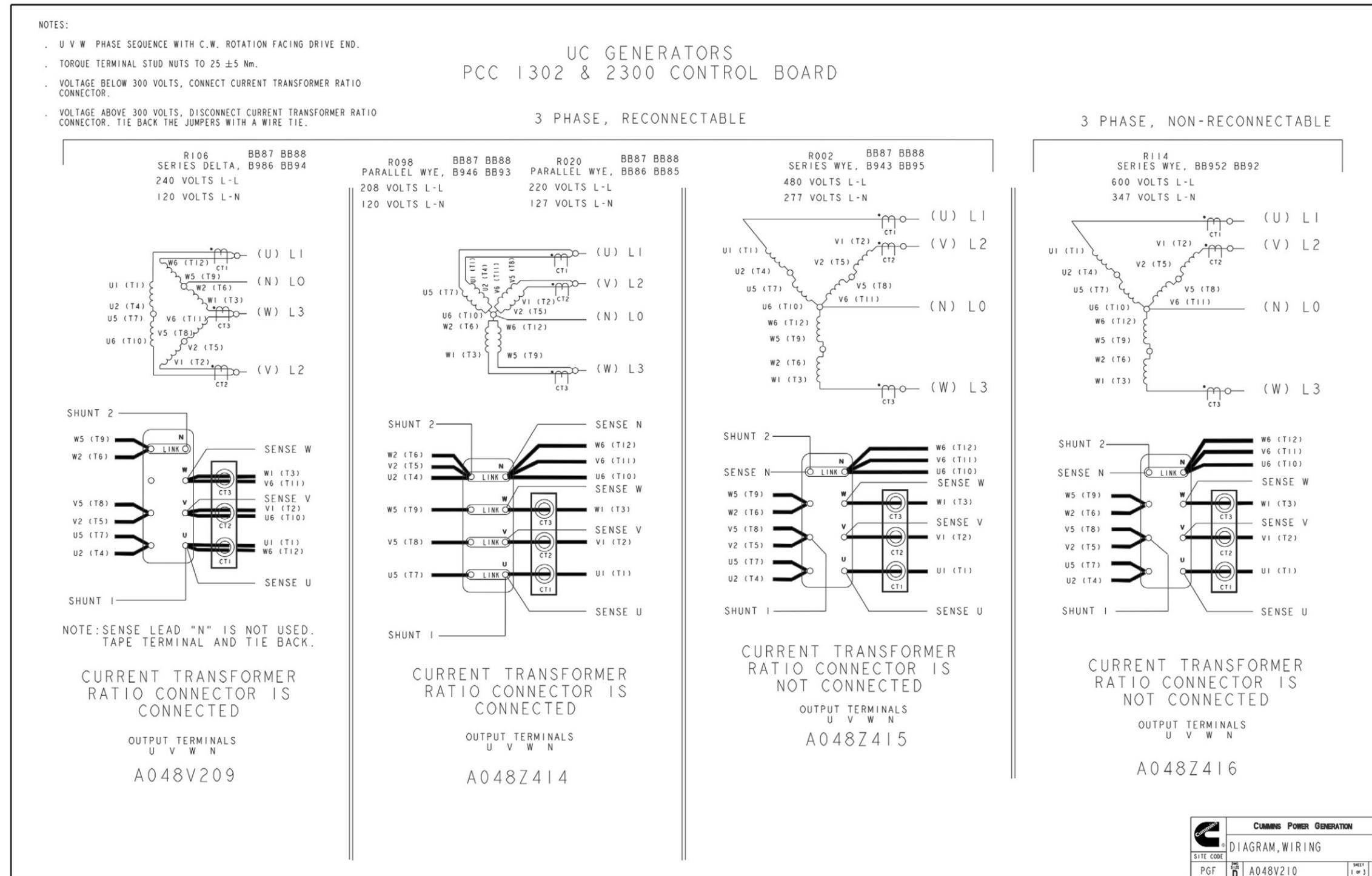
FIGURE 116. RECONNECT DRAWING FOR UC ALTERNATOR (SHEET 1 OF 3)
