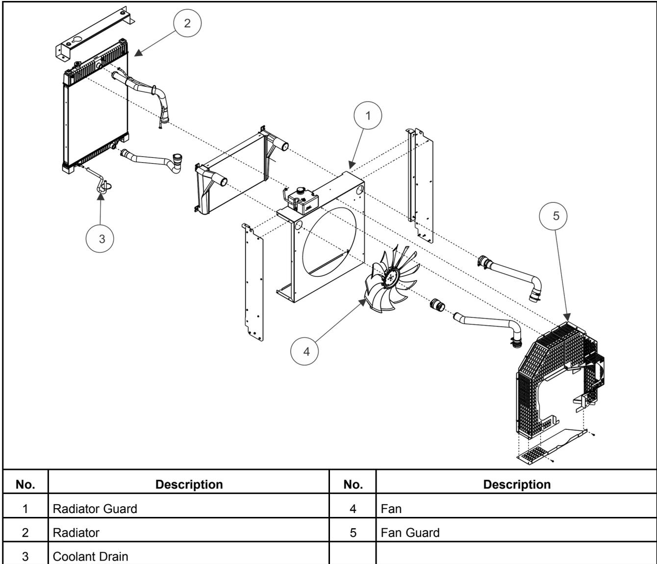
FIGURE 44. COOLING SYSTEM FOR GENERATOR SET WITH QSJ8.9G ENGINE
