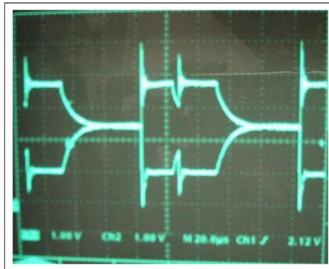
**FIGURE 32. CAN DATALINK: BAD SIGNAL**
