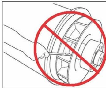
**FIGURE 64. DO NOT ROTATE THE ALTERNATOR ROTOR USING THE COOLING FAN VANES.**
