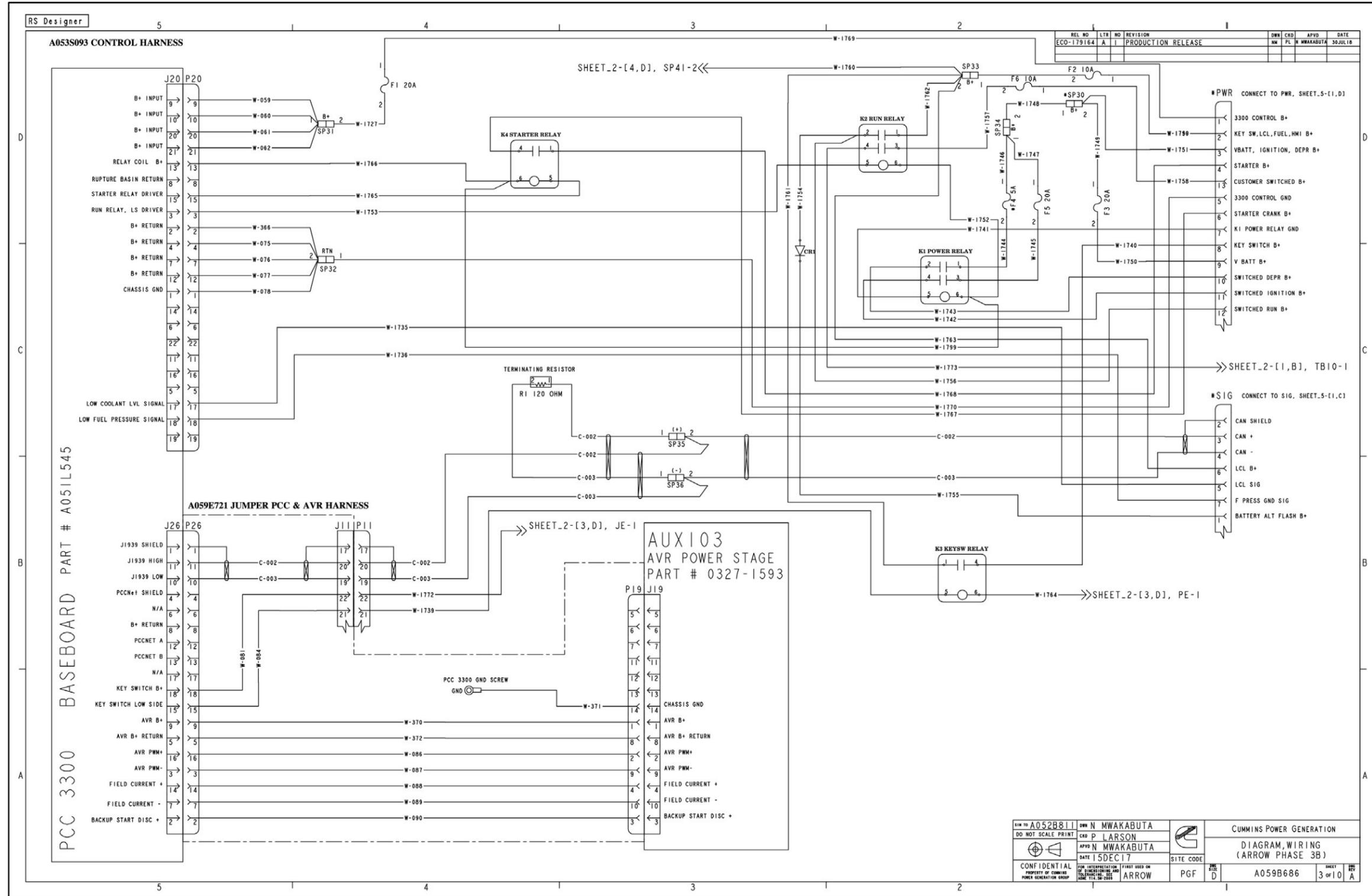
FIGURE 101. WIRING DIAGRAM PC 3.3 (SHEET 3 OF 10)
