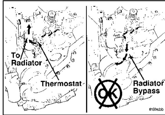
**FIGURE 68. ALWAYS USE THE CORRECT THERMOSTAT**
