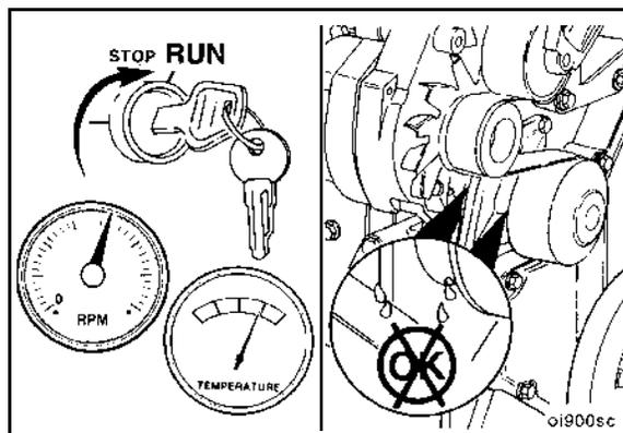
**FIGURE 52. CHECK FOR COOLANT LEAKS**
