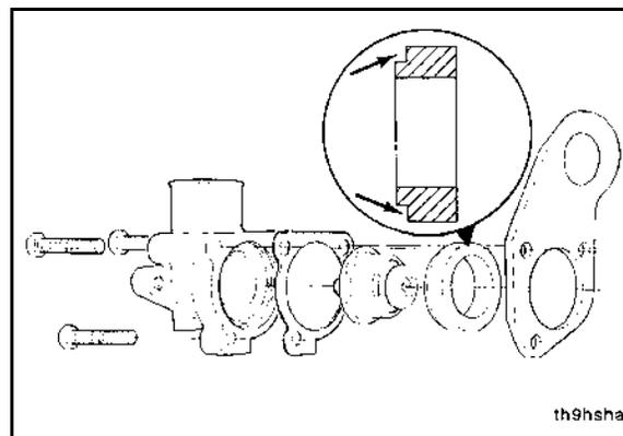
**FIGURE 69. REMOVE THREE CAPSCREWS, THE THERMOSTAT HOUSING, LIFTING BRACKET, THERMOSTAT, AND THERMOSTAT SEAL**
