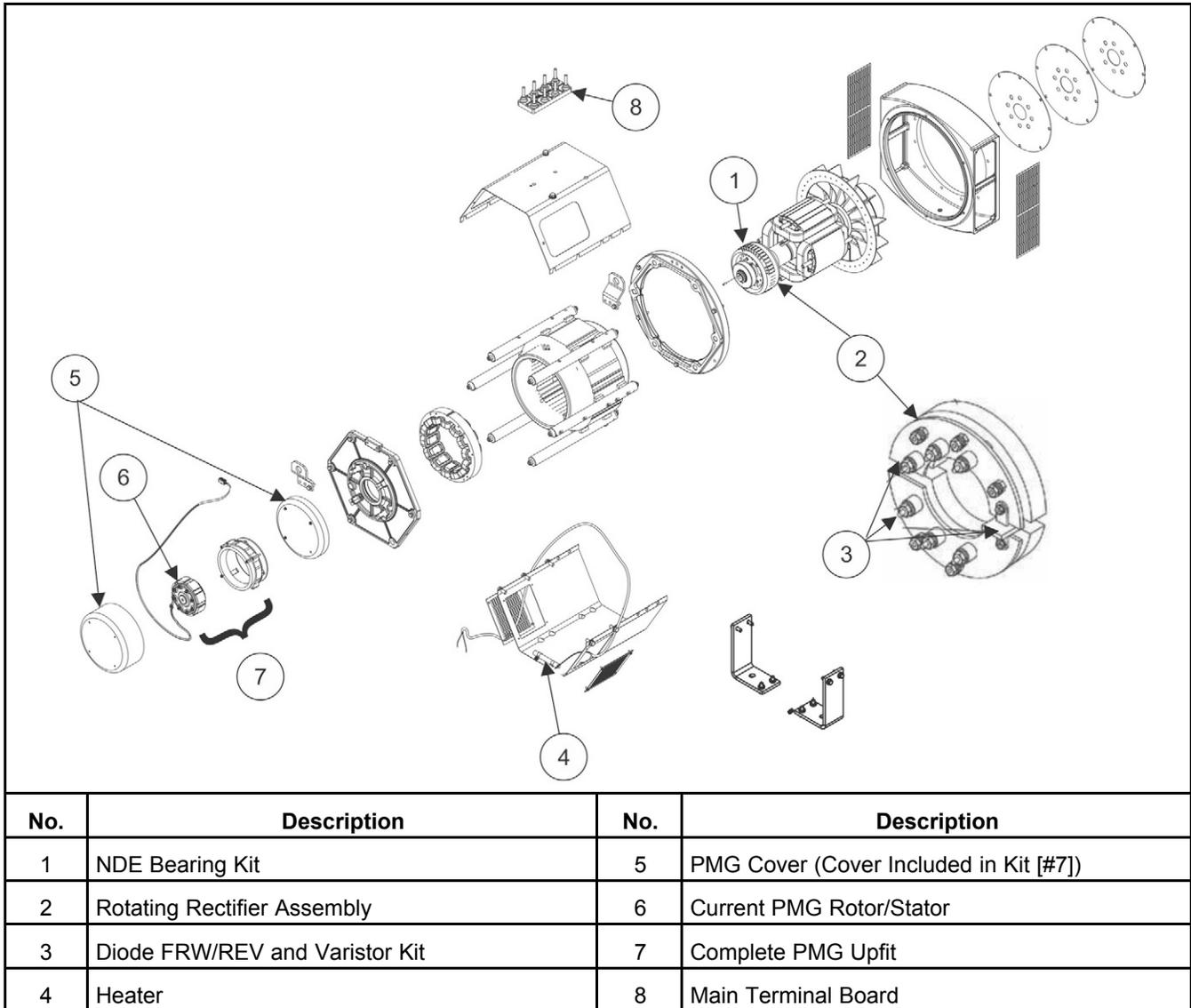
FIGURE 67. UC SINGLE BEARING ALTERNATOR PARTS
