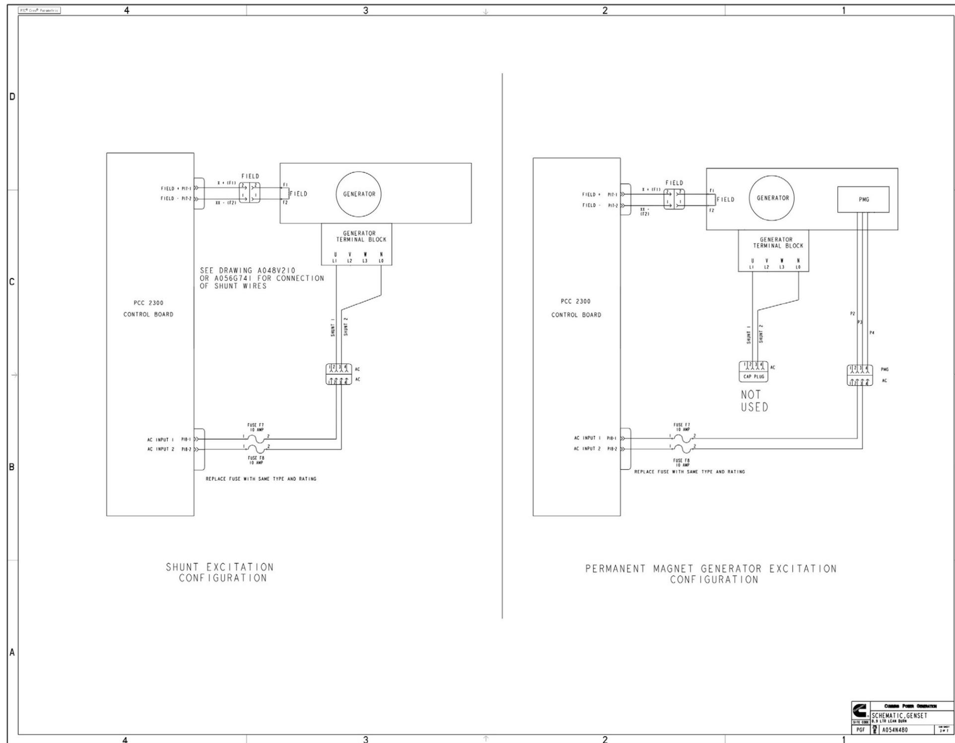
FIGURE 94. WIRING DIAGRAM PC 2.3 (SHEET 3 OF 7)
