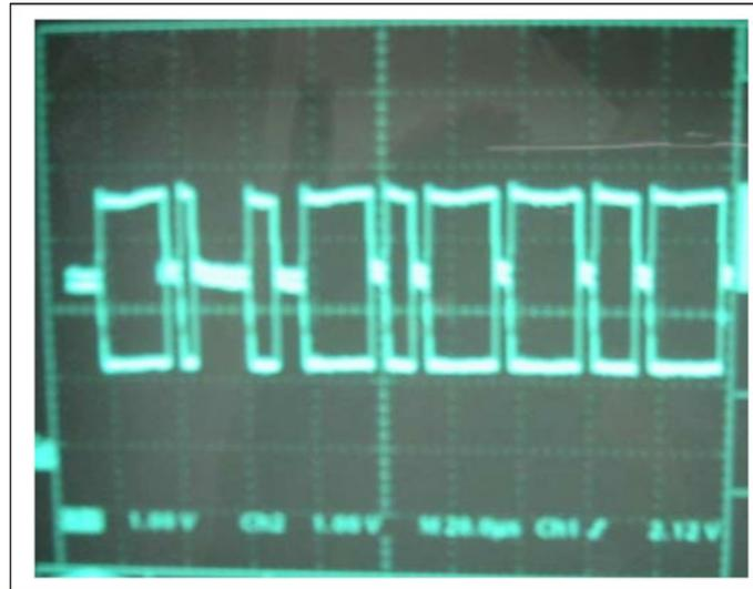
**FIGURE 31. CAN DATALINK: GOOD SIGNAL**
