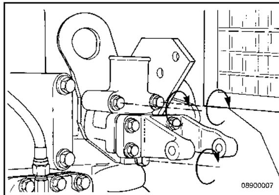
**FIGURE 73. INSTALL THE THERMOSTAT, THERMOSTAT SEAL, THERMOSTAT HOUSING, GASKET, LIFTING BRACKET, AND THREE CAPSCREWS**
