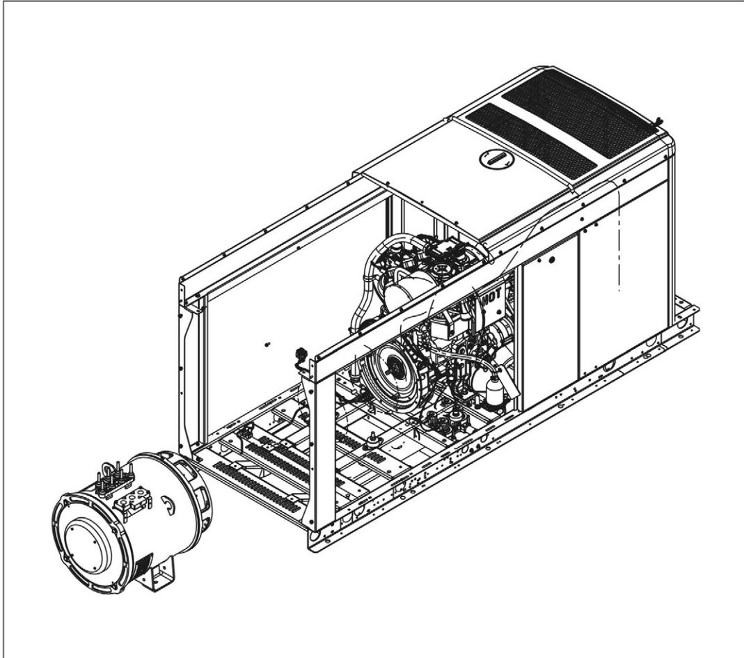
**FIGURE 63. MOVING THE ALTERNATOR EXAMPLE**
