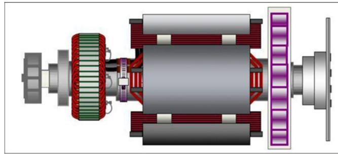
**FIGURE 65. SINGLE BEARING ALTERNATOR ROTOR SHOWING COUPLING DISCS BOLTED TO DRIVE END COUPLING HUB (AT RIGHT)**
