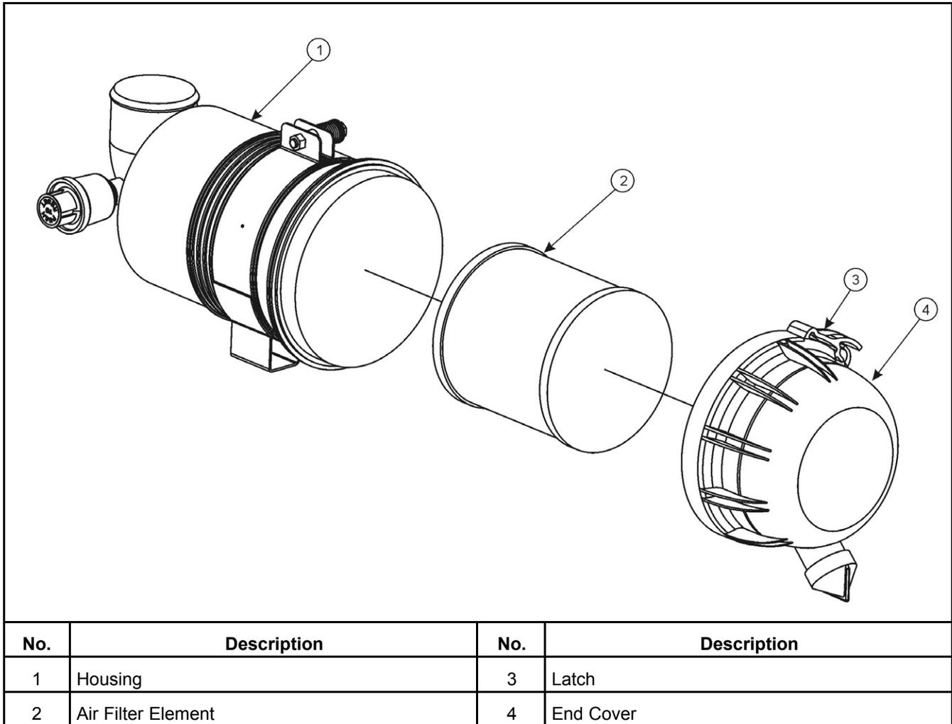
FIGURE 15. EXAMPLE OF HEAVY DUTY AIR CLEANER
