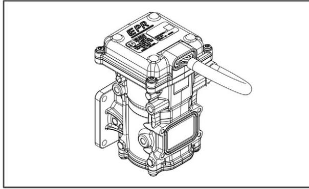
**FIGURE 41. DIRECT ACTING PRESSURE REGULATOR (DEPR)**
