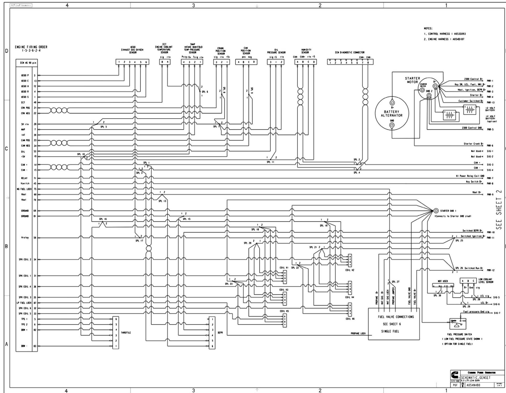
FIGURE 92. WIRING DIAGRAM PC 2.3 (SHEET 1 OF 7)
