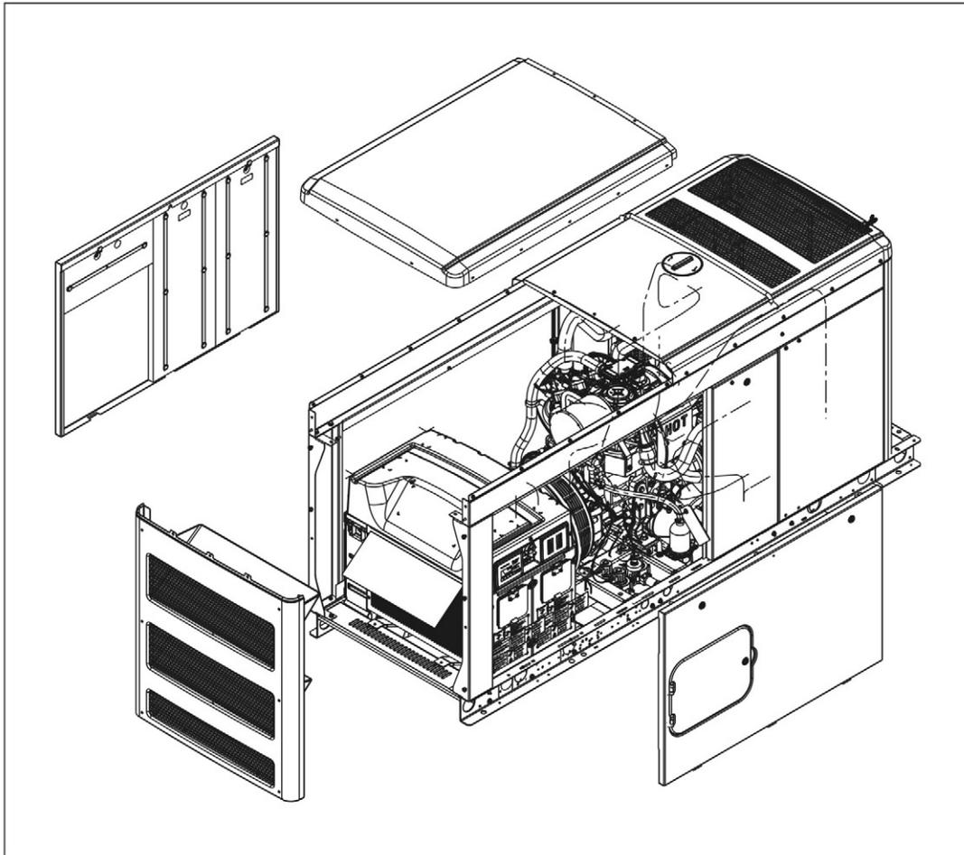
**FIGURE 58. REMOVE ENCLOSURE EXAMPLE**
