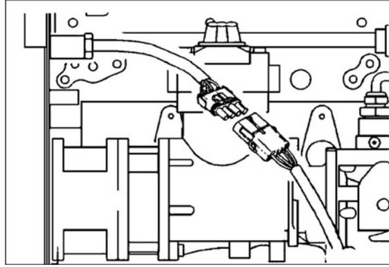
**FIGURE 16. CHECK HARNESS CONNECTIONS**
