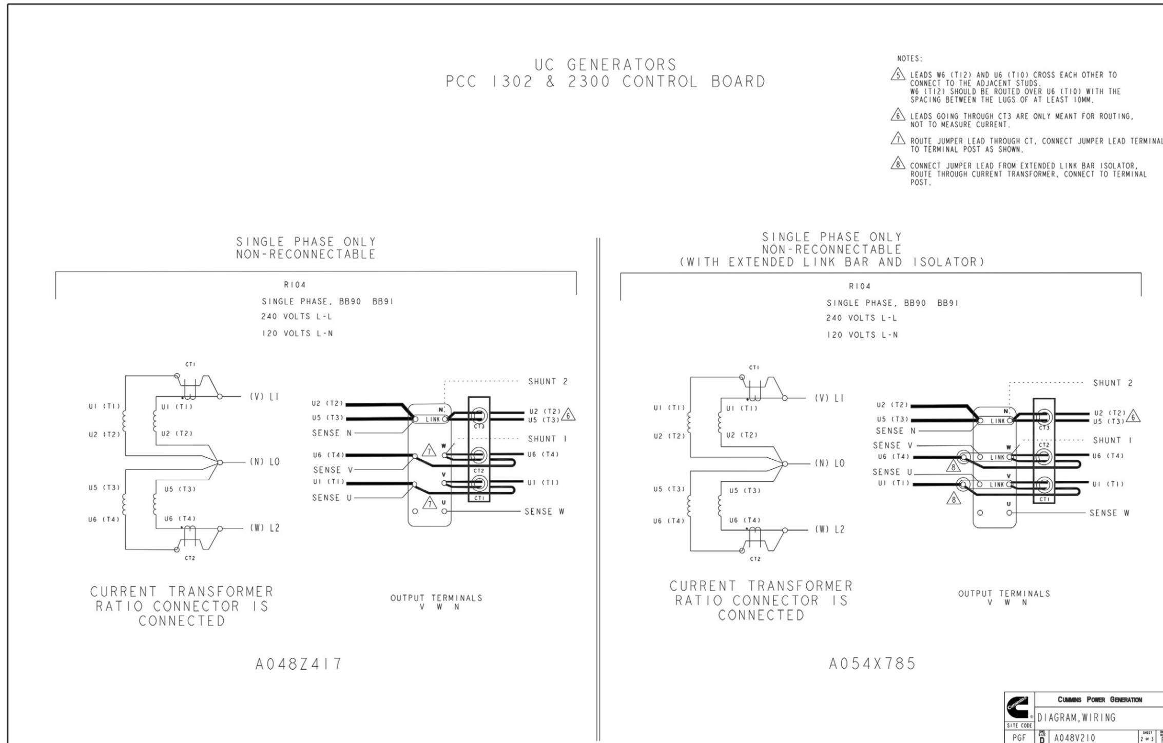
FIGURE 117. RECONNECT DRAWING FOR UC ALTERNATOR (SHEET 2 OF 3)
