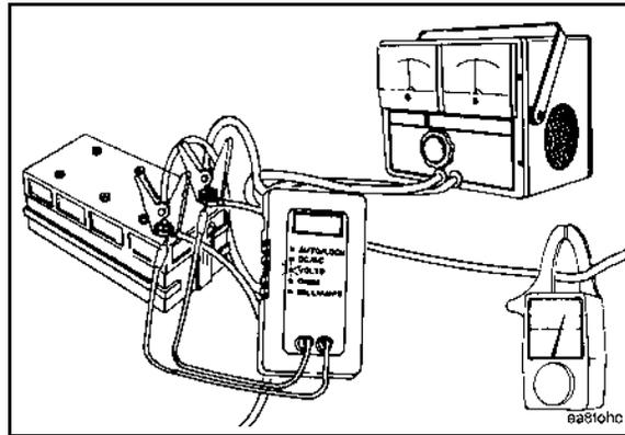
**FIGURE 83. CONNECT A CARBON PILE LOAD**
