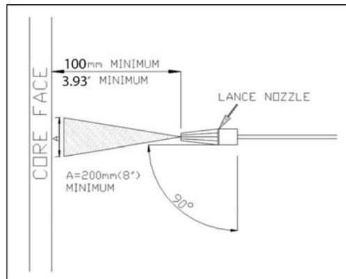
FIGURE 8. PRESSURE WASHER NOZZLE POSITIONING
