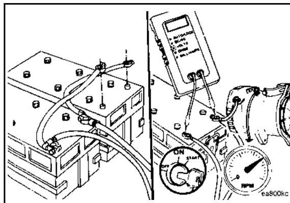
**FIGURE 84. DISCONNECT BATTERY CABLES; MEASURE THE ALTERNATOR VOLTAGE OUTPUT**
