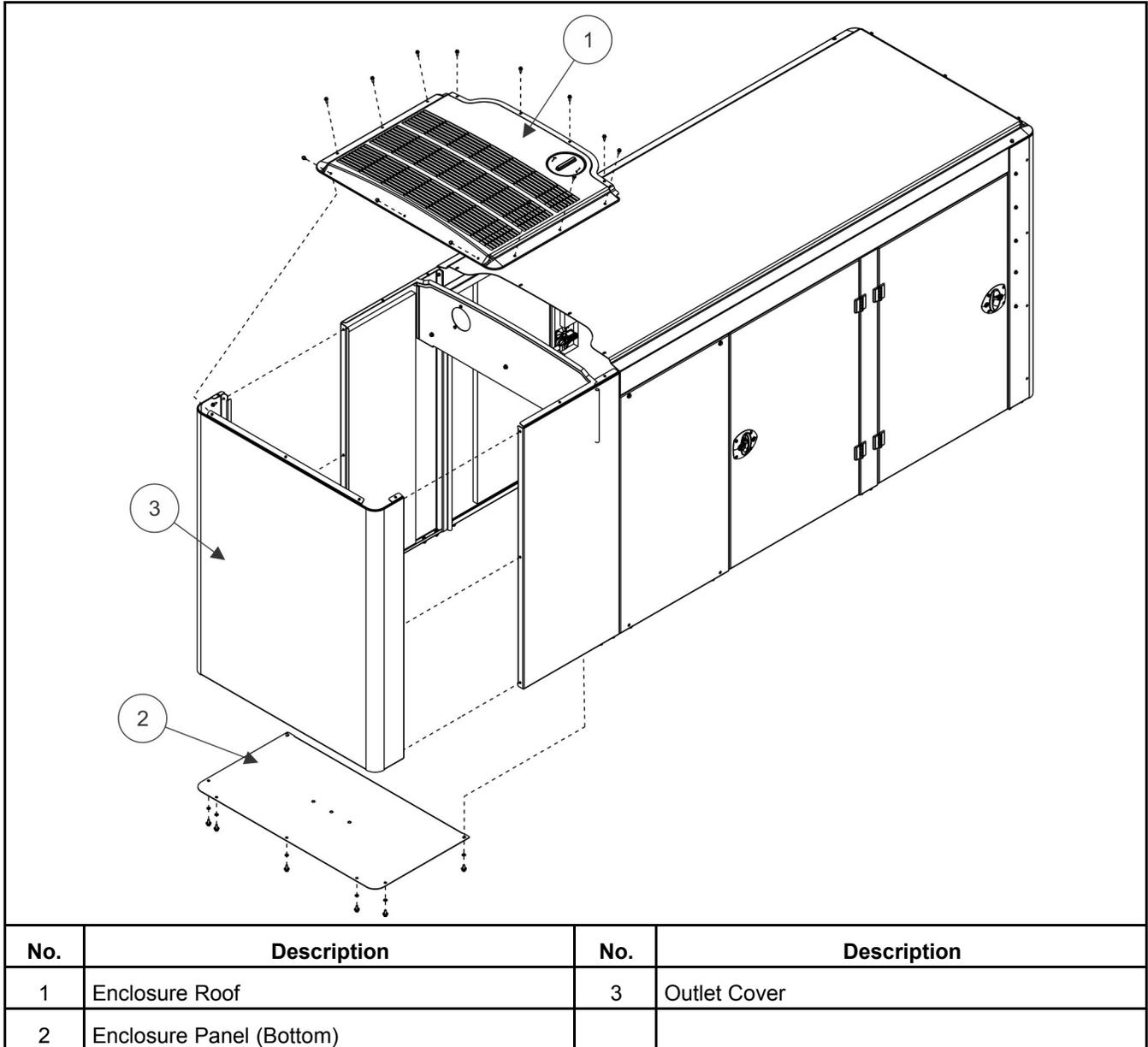
**FIGURE 55. ENCLOSURE REMOVAL**
