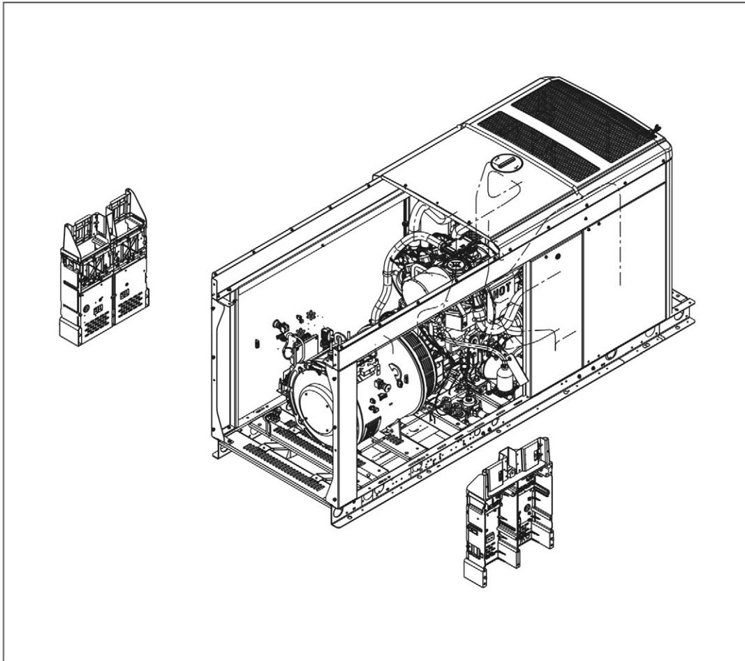
**FIGURE 59. REMOVE TERMINAL BOX MOUNTING BOLTS EXAMPLE**
