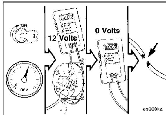
**FIGURE 82. CHECK FOR OPEN CIRCUITS**
