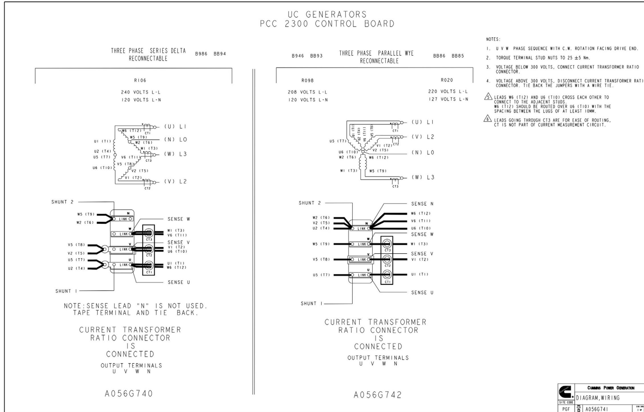
FIGURE 119. RECONNECT DRAWING FOR UC ALTERNATOR (SHEET 1 OF 3)
