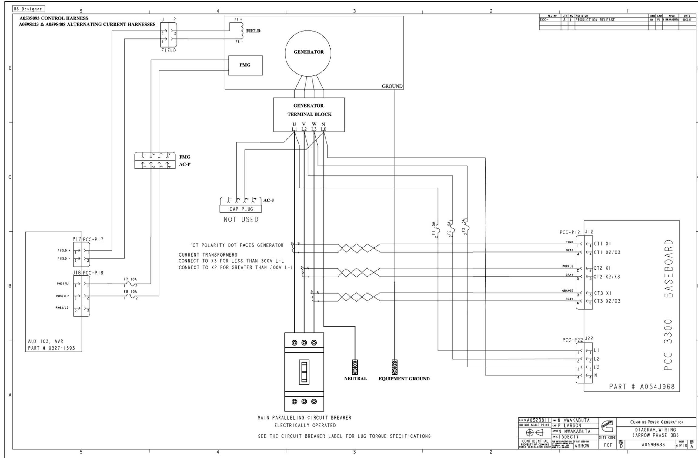
FIGURE 104. WIRING DIAGRAM PC 3.3 (SHEET 6 OF 10)
