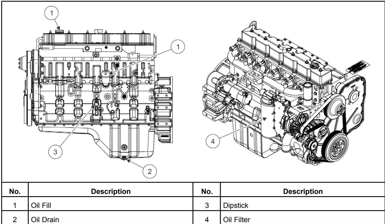
**FIGURE 2. ENGINE OIL COMPONENTS**
