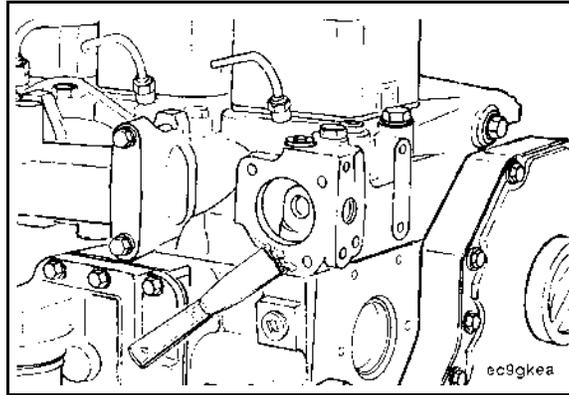
**FIGURE 70. CLEAN THE MATING SURFACES**
