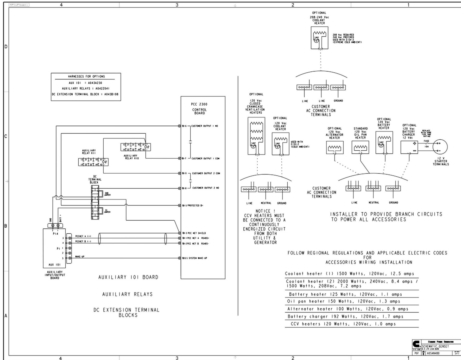
FIGURE 96. WIRING DIAGRAM PC 2.3 (SHEET 5 OF 7)
