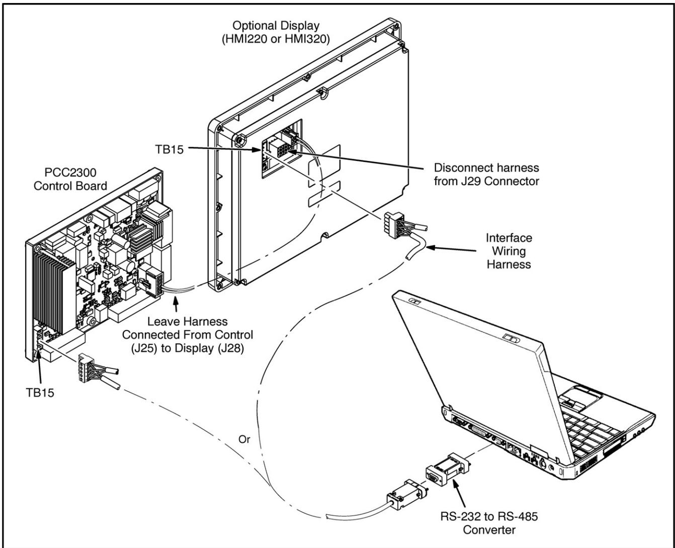
**FIGURE 35. KIT INSTALLATION FOR PCC2300 WITH HMI220 OR HMI320 DISPLAY**
