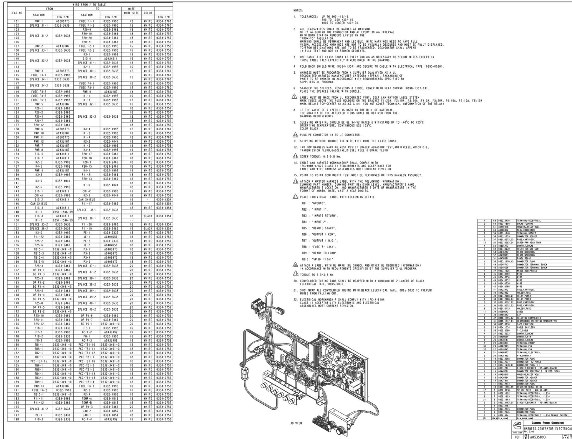
FIGURE 112. CONTROL BOX HARNESS DIAGRAM (SHEET 1 OF 4)
