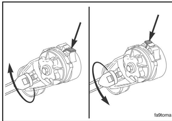
**FIGURE 3. LIFT THE TENSIONER TO REMOVE THE BELT**
