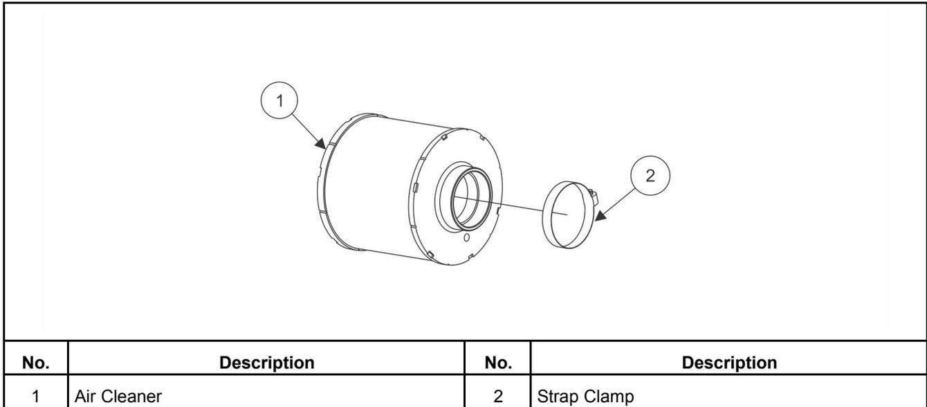
FIGURE 14. EXAMPLE OF NORMAL DUTY AIR CLEANER
