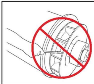
**FIGURE 61. DO NOT ROTATE ROTOR USING FAN**
