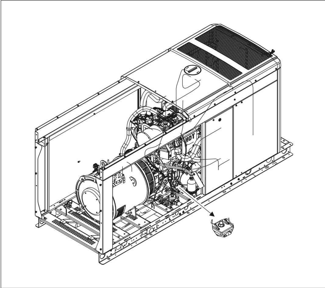
**FIGURE 60. REMOVE AND SECURE THE ALTERNATOR (WITH DETAIL) EXAMPLE**
