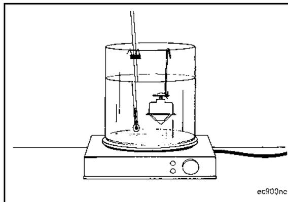
**FIGURE 71. SUSPEND THE THERMOSTAT AND THERMOMETER IN WATER**
