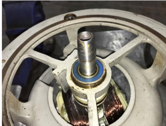
**FIGURE 65. ROTOR AND CRANKSHAFT**
